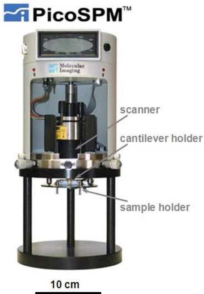
Figure 2.1: The PicoSPM Atomic Force Microscope in our laboratory.
